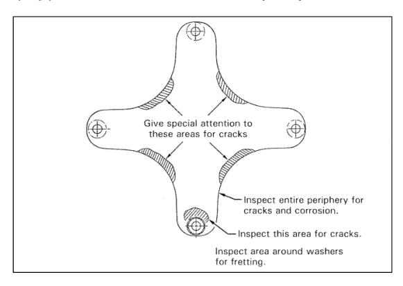
(ii) Visually inspect yoke P/N C907–1 or C907–2, as applicable to your model helicopter, and yoke P/N C908–1, for any cracks, corrosion, and fretting. If there is any crack, corrosion, or fretting, before further flight, remove the yoke from service and replace it with an airworthy yoke, and torque each newly-installed bolt, nut, and palnut using the torque value information in Appendix 1 to this AD.
