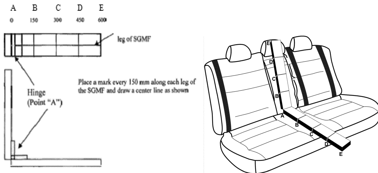
Figure 1. SGMF sketch (left), SGMF positioned in a vehicle rear (center) seating position.
