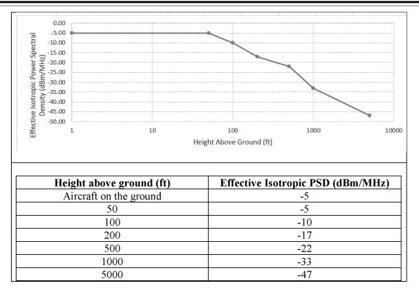
(ii) Tolerance to radio altimeter interference, for the spurious emissions (4.2– 4.4 GHz), at or above the PSD curve threshold
