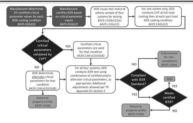
Figure II-1: CCE Process Diagram for VRF Multi-split Systems
