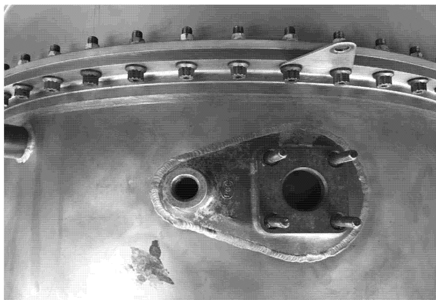
Figure 2 to Paragraph (h) of this AD. Combustion Chamber Case Assembly with One-Piece Bleed Pad with P3 Boss
