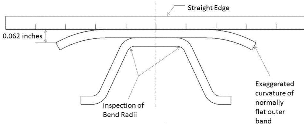
Figure 1 to paragraphs (k)(1)(iii) and (v) of this AD: Cross section of v-band coupling
