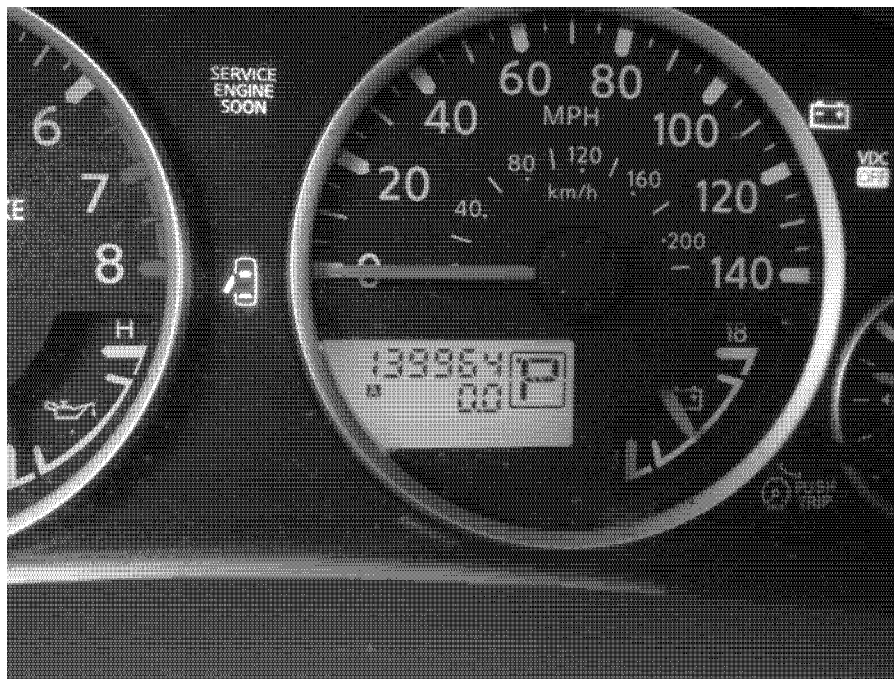
Photo 4 – Subject vehicle MIL - "Service Engine Soon"
