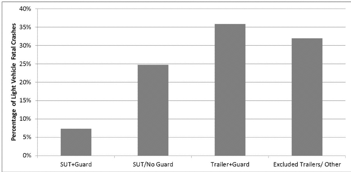
Figure 2. Percentage of light vehicle fatal crashes into the rear of SUTs and trailers (2008-2009 TIFA UMTRI Study)
