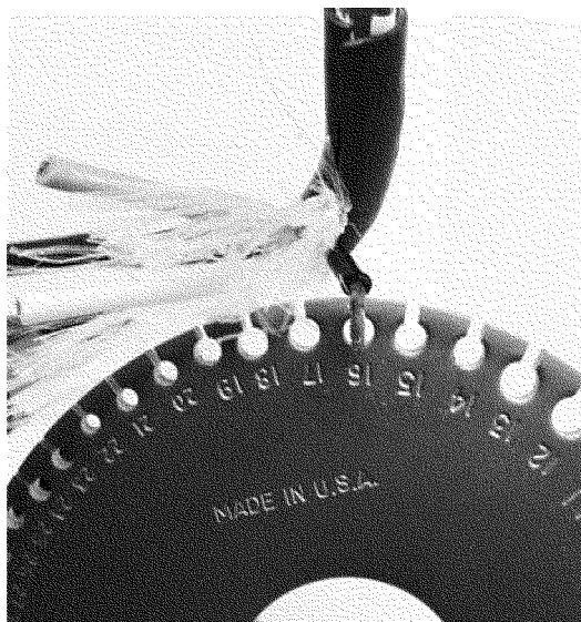
Picture 2: Measuring Wire Size
