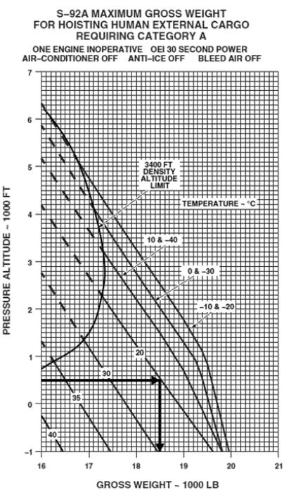
NOTE 1: THIS CHART DEPICTS THE GROSS WEIGHT, PRESSURE ALTITUDE, TEMPERATURE COMBINATION WHERE OEI HOGE CAPABILITY EXISTS USING 30 SECOND OEI POWER WITH A 60 SHP MARGIN.
