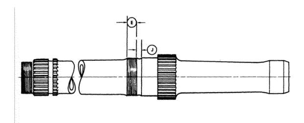
(2) If there is a crack, pitting, or corrosion, before further flight, replace the mast with an airworthy mast.
