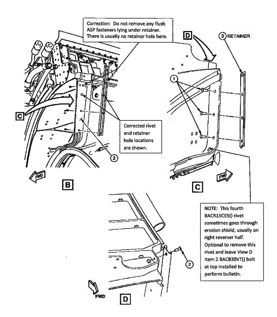
Figure 4, Installation of the New Bracket behind the Retainer Support on the Right Thrust Reverser Half
