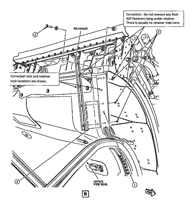
Figure 3, Fastener Removal of the Retainer Support on the Right Thrust Reverser Half
