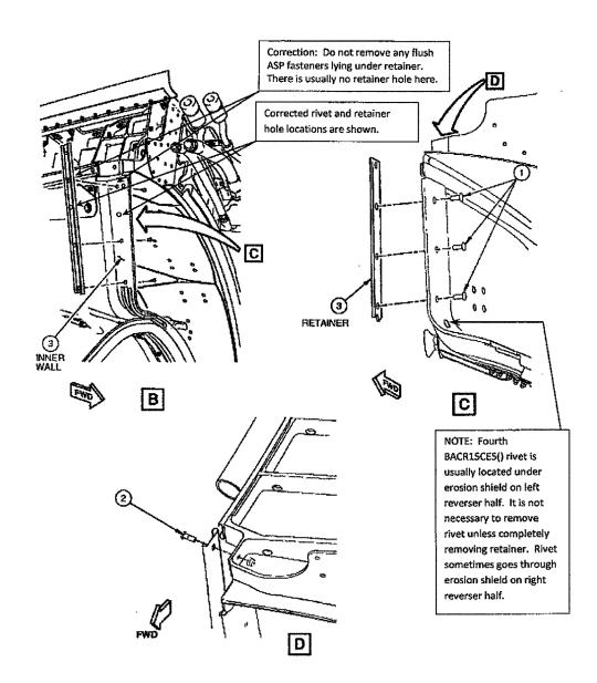
Figure 2, Installation of the New Bracket behind the Retainer Support on the Left Thrust Reverser Half
