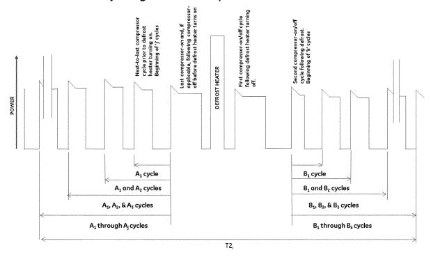
Figure 1 Note: The average temperatures of the compartments for compressor cycles A<sub>1</sub> through A<sub>i</sub> shall be within 0.5 °F (0.3 °C) of their temperature averages for the first part of the test. Likewise, the average temperatures of the compartments for compressor cycles B<sub>1</sub> through B<sub>k</sub> shall be within 0.5 °F (0.3 °C) of their temperature averages for the first part of the test.
