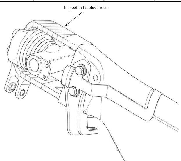
(4) If there is a crack, or if there is damage that exceeds the limits of the applicable maintenance manual, before further flight, replace the T/R blade with an airworthy T/ R blade.
