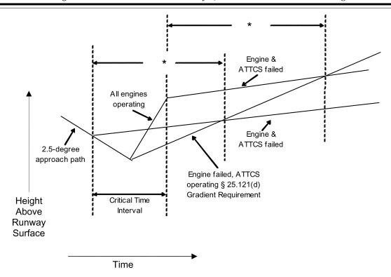
\* The engine-and-ATTCS failed time interval must be no shorter than the time interval from the point of simultaneous engine and ATTCS failure to a height of 400 feet used to comply with I25.2(b) for ATTCS use during takeoff.
