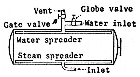
(1) Size of vent and vent valve. For retorts less than 15 feet (4.6 meters) in length, 2 inches (5.1 centimeters); for retorts 15 feet (4.6 meters) and over in length, 2.5 inches (6.4 centimeters).
