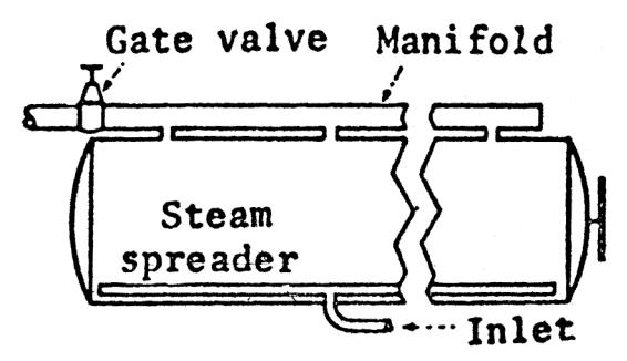
(1) Specifications. One 1-inch (2.5 centimeters) vent for every 5 feet (1.5 meters) of retort length; and vents not over 2.5 feet (76 centimeters) from ends of retort. Size of manifold—for retorts less than 15 feet (4.6 meters) in length,
