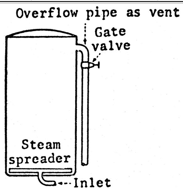
(1) Specifications. A 1.5-inch (3.8 centimeters) overflow pipe equipped with a 1.5-inch (3.8 centimeters) gate or plug cock valve and with not more than 6 feet (1.8 meters) of 1.5-inch (3.8
