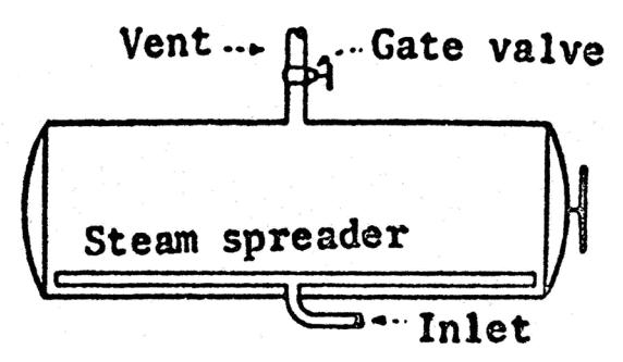
(1) Specifications. A 2.5-inch (6.4 centimeters) vent equipped with a 2.5-inch (6.4 centimeters) gate or plug cock valve and located within 2 feet (61 centimeters) of the center of the retort.
