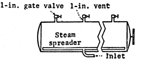
(1) Specifications. One 1-inch (2.5 centimeters) vent for every 5 feet (1.5 meters) of retort length equipped with a gate or plug cock valve and discharging to atmosphere; end vents not more than
