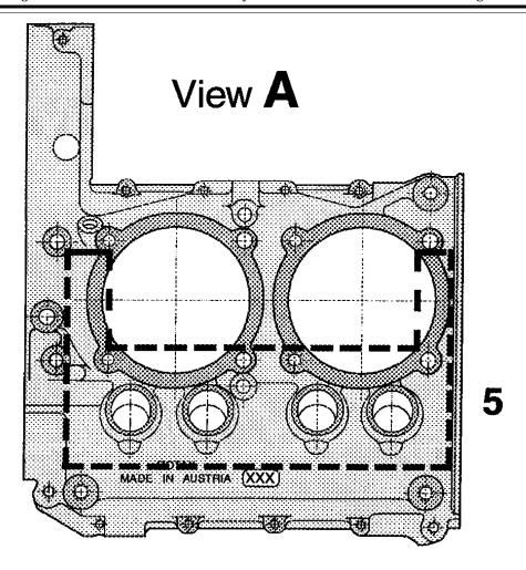
Figure 2. Engine Crankcase Inspection Areas – View A
