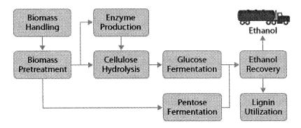
While this diagram shows the production of ethanol from cellulosic biomass, it is possible to use the same process to produce other fuels or specialty chemicals using different biological organisms.
