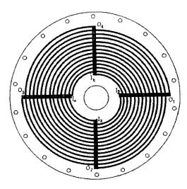
The support compactly holds spirally wound plastic tubing at a desired spiral pitch without connection. When mounted on the existing high-speed countercurrent chromatographic centrifuge, it will produce separation of bioactive compounds including proteins, nucleic acids, polysaccharides, and small molecular weight compounds from natural products without loss of samples in the separation column.
