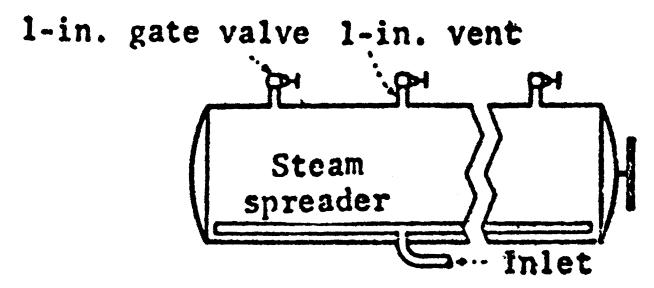
Specifications. One 1-inch (2.5 centimeters) vent for every 5 feet (1.5 meters) of retort length equipped with a gate or plug cock valve and discharging to atmosphere; end vents not more than 2.5 feet (76 centimeters) from ends of retort.
