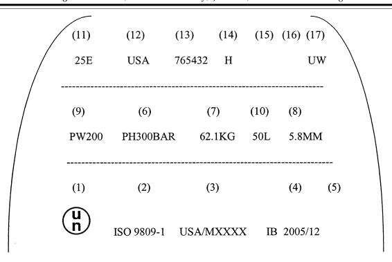
(q) Other markings. Other markings are allowed in areas other than the side wall, provided they are made in low stress areas and are not of a size and depth that will create harmful stress concentrations. Such marks must not conflict with required marks.
